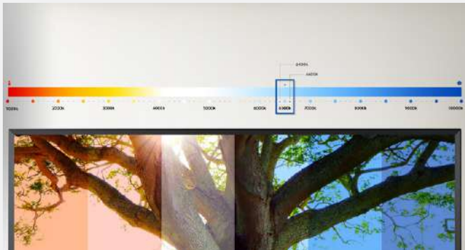
Figure 7. Three options enable the user to adjust the display's white balance.
